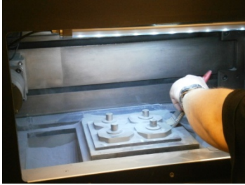
Cleaning off extra powder from finished build in DMLS machine
