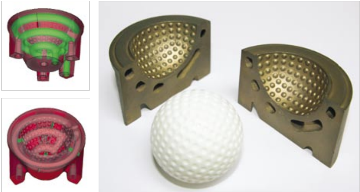
Figure 4 Golf Ball blow-mould Left: Conformal cooling Middle: Venting channels (Green) Right: DirectTool cavity Courtesy: Es-Tec, DemoCenter
